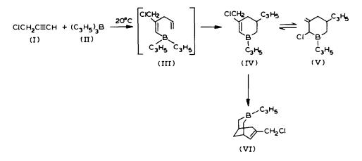
When heated at  $120-130^{\circ}$ C for 45 min, the mixture forms the bicyclic compound VI along with 3-5% of the isomeric 6-chloro-7-methylene-3-allyl-3-borabicyclo[3.3.1]nonane (VII) [5].
